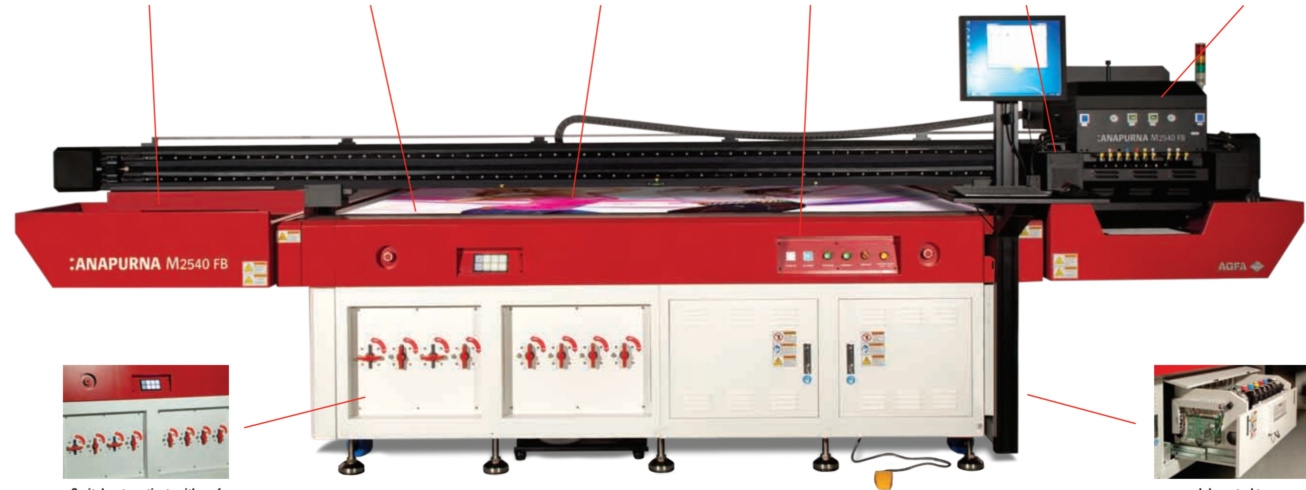
Switches to activate either of the 8 vacuum compartments
