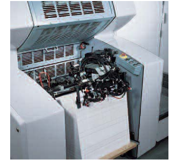
Quality begins at the feeder with constant register accuracy based on double-sheet control, a suction tape feed board and combined lifting/forwarding suckers
